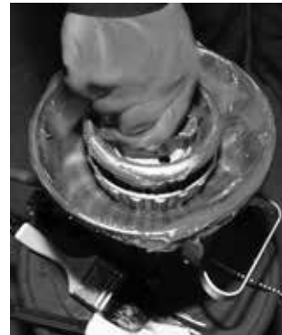
Fig. 24. Mechanical grease packer.
