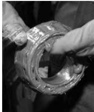
Fig. 23. Grease can easily be packed by hand.
